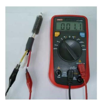
Sensor test— use an ohmmeter to check sensor resistance, resistance value at room temperature should be around 1 ohms. Sensor is polarity sensitive, red wire for positive probe, and yellow wire for negative/ground probe.
