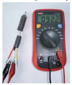
Heating element test -use an ohmmeter to check heater resistance, resistance values should be around 90 ohms.
